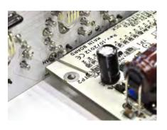
10.: Attach the tube board to the main board. Now solder with a piece of (cutted) wire a connection between pin "HV" of the tube board to "TP2" on the main board. This will feed the 170V, which are necessary to power the neons, to the tube board.
