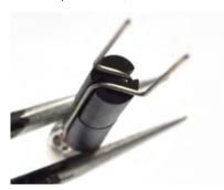
5.: Bend the neon's wires as shown in the picture. Do not make any short ciruit.
