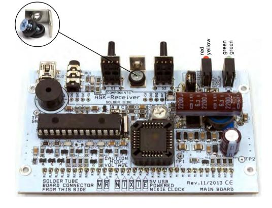
Now connect the PCB to an USB power supply and check if something strange will happen; e.g. a parts runs hot. If everything is allright we will do follwing some voltage checkings: Please check the voltages on the PIC's socket pins with a multimeter. **Put the negative probe (black) on TP3**: left hand from the buzzer. Put the positive probe (red) on the socket pins.
