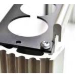
Next pick up both reinforcement profiles and att ach them to the enclosure. To enable this you need to bend the (only with one screw fixed) right hand profile a little bit.
