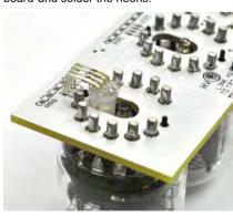
8.: Fit the LEDs to the board and solder them. Use as less solder tin as possible as the spacing between the LED pins is very small.
