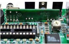
Simply fit the module onto the mainboard and solder the 8 pins. Pay attention for correct orientation (see pictures).
