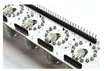
9.: Fit the 32-pin header and the resistor arrays (the "polarity" is negligable) from solder side and solder them.
